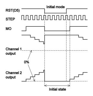
When the reset bit in the serial data, D5 (100, \*\*, D5, \*\*), is set to 0, the output goes to the initial state at the rise of STB and the MO output goes low.
